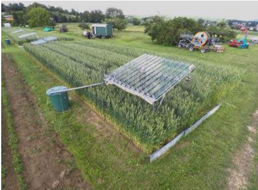
Rain-out shelters in the DOK trial to simulate the expected drought scenarios
